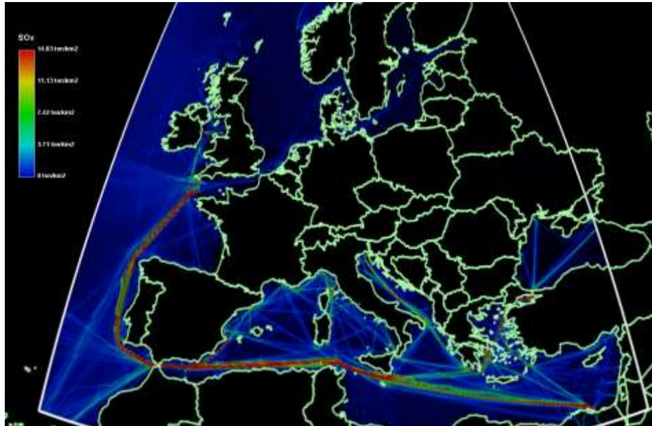
Figure 4 Europe-region level, SO 2 annual average concentration, exclusively GNFR7 water shipping navigation transport sector.
