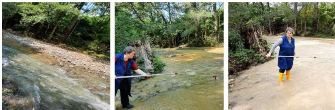
(SS9) Water sampling on Veliki Pek – tourist site Ujevac (the influence of tailings)
