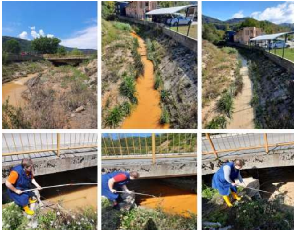
(SS3) Water sampling on Mali Pek after inflow of drainage water from the North Mining District dump and wastewater from grinding
