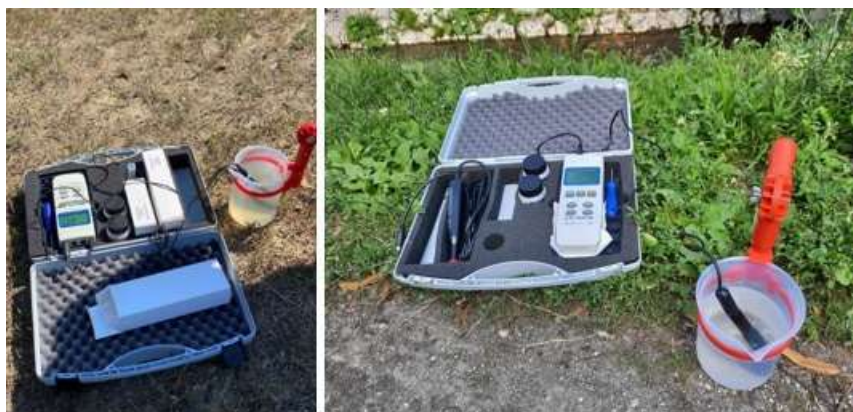
Figure 2. Determination of parameters using a multi-parameter measuring instrument
